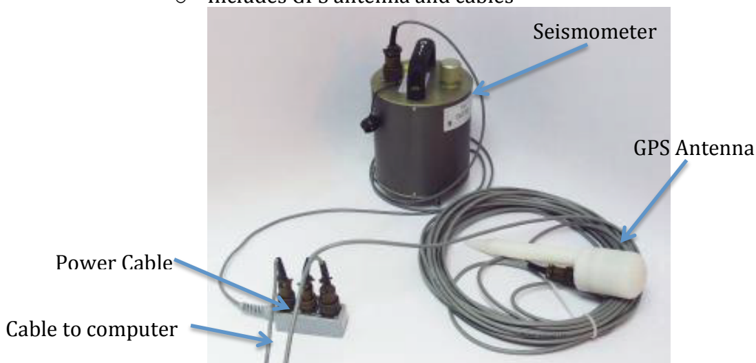
Figure 1: Seismometer with GPS antenna and cables
